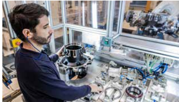
Preset hub assemblies control area.
